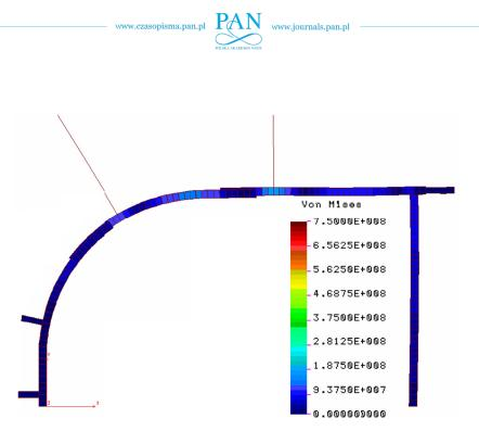
Fig. 8. Distribution of the von Misses stresses in the 3.3 model of the LPrO frame support with diagonally located anchors and anchored canopy (model designation consistent with table 1 – frame with two bolts, C support stiffness modulus  $K_C = 100$  kN/m)
