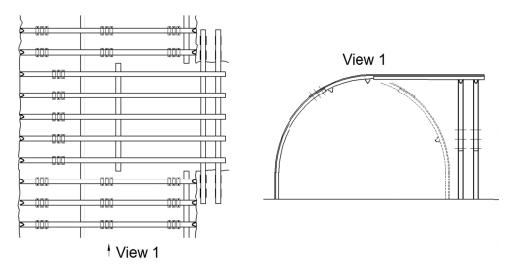
Fig. 3. General diagram of the support of the support of three-way intersection of workings
