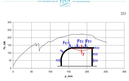
Fig. 10. Characteristics of the ŁPrOJ6.2/4.0/V36 support frame tested in a stiffened state Fc – load of the arch support (Fc = Fc1 + Fc2 + Fc3), y – deflection of the arch (in midpoint of canopy)
