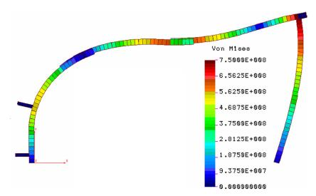
Fig. 6. Distribution of the von Misses stresses in the 1.3 model of the LPrO frame support (model designation consistent with table 1 – frame without bolts, C support stiffness modulus  $K_C = 100$  kN/m)
