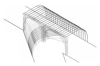
Fig. 4. Example of the support of underground workings secured by arch-rectangular support (thick lines)
