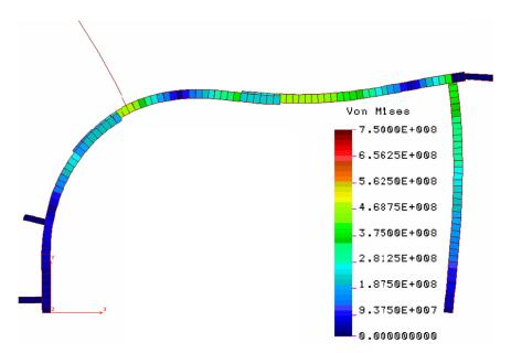
Fig. 7. Distribution of the von Misses stresses in the 2.3 model of the LPrO frame support with diagonally located anchors (model designation consistent with table 1 – frame with one bolt, C support stiffness modulus  $K_C = 100$  kN/m)
