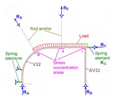
Fig. 5. The basic scheme of boundary conditions and load of the analysed frame support
