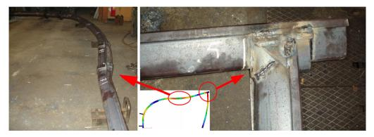
Fig. 9. Arch-rectangular support after tests and comparison with results of numerical modling. Deformation of the canopy (on the left) and deformation of the canopy and prop connection (right)
