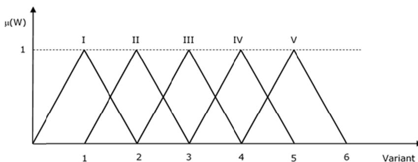
Fig. 1. Membership functions for FSDR system output values
