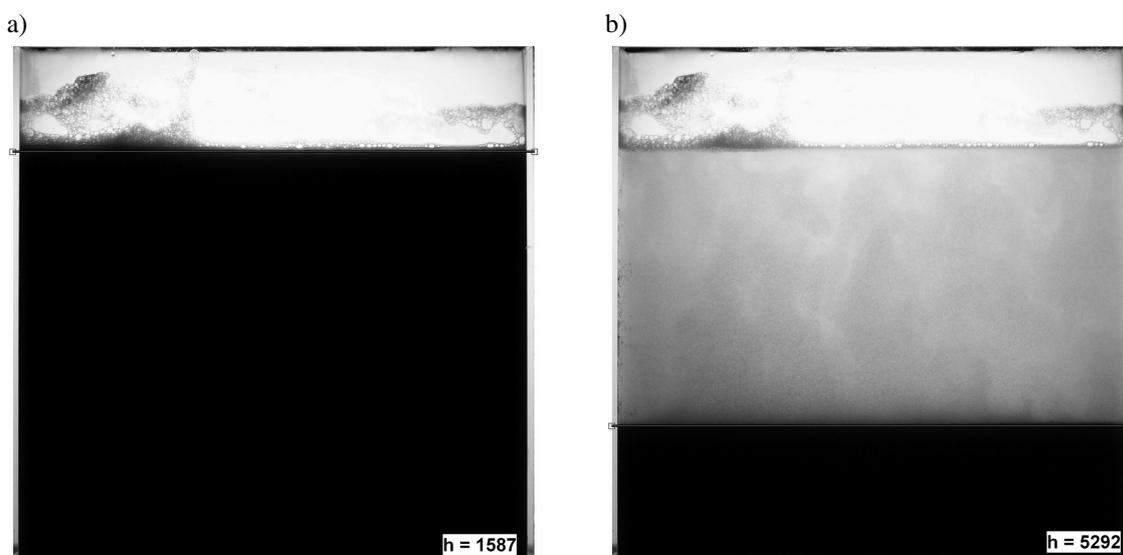
Fig. 10. Images of the suspension of dewatering granules at their concentration of about 14 vol% in the beet juice after carbonation I, with lines indicating the position of the upper border of discontinuity: a) at the process initiation, b) after 105 seconds of the process duration
