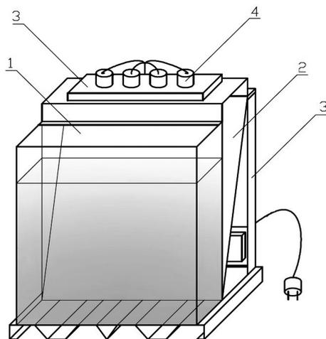
Fig. 1. Scheme of the experimental setup; 1 – glass container, 2 – light reflecting surface, 3 – cover, 4 – halogen bulbs with casings
