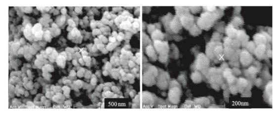
Fig. 2. Scanning Electron Microscopy (SEM) images of synthesized zinc nanoparticles in different zoom
