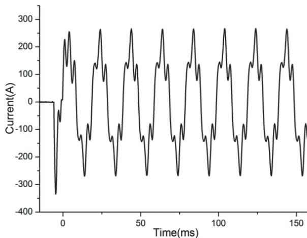
Fig. 8. Direct grounding current waveform of substation D
