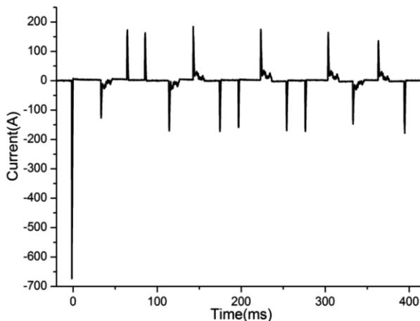
Fig. 7. Arc grounding current waveform of substation J
