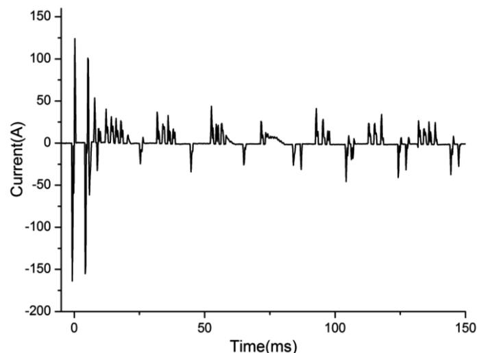
Fig. 3. Arc grounding current waveform of substation I
