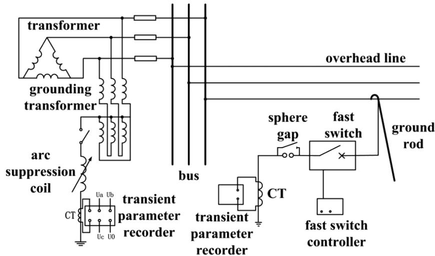
Fig. 2. Schematic diagram of single phase grounding test using fast switch
