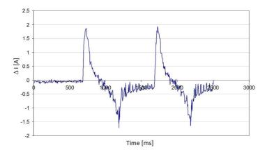
Figure 10: Current difference between load and response signal of two Nexa modules connected in parallel for semi-sinusoidal load signal with amplitude  $15~\mathrm{A}$  and period  $1000~\mathrm{ms}$ .
