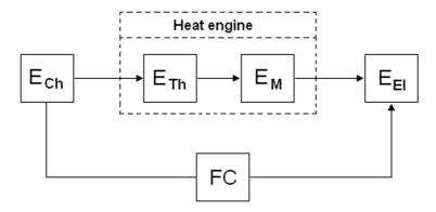
Figure 1: Direct energy conversion with fuel cell in comparison to conventional indirect technology: FC - fuel cell, E<sub>El</sub> - electrical energy (electricity), E<sub>M</sub> - mechanical energy,  $E_{\rm Ch}$  – chemical energy,  $E_{\rm Th}$  – thermal energy.
