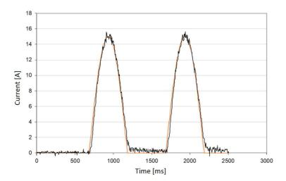
Figure 9: Current response of the two Nexa power modules for semi-sinusoidal load signal with amplitude  $15~\mathrm{A}$  and period  $1000~\mathrm{ms}$ .
