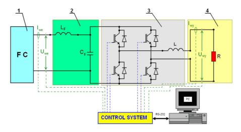
Figure 4: Scheme of the PEMFC system: 1-FC module, 2-filter, 3-electronic load system, <math>4-resistive load.
