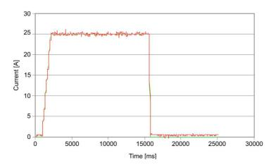
Figure 11: Current response of the two Nexa modules for trapezoidal load signal with an amplitude  $25~\mathrm{A}$ , period  $15000~\mathrm{ms}$  and ramp  $1400~\mathrm{ms}$ .
