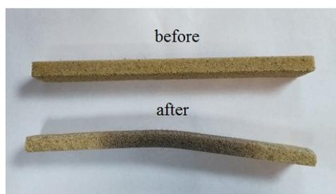
Fig. 1. Deformation of moulding sand with the geopolymer binder Geopol<sup>®</sup> during hot-distortion tests [33]
