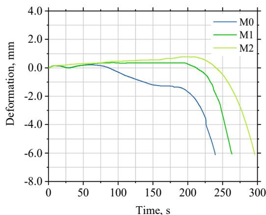
Fig. 2. Dependence of the thermal deformation of moulding sands with the geopolymer binder Geopol<sup>®</sup> on the heating time
