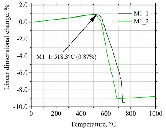
Fig. 5. Dilatometric curves for moulding sand M1
