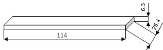
Fig. 2. Hot-distortion sample[16]
