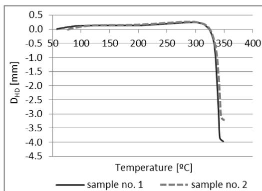
Fig. 6. Thermal deformation of the sample as function of temperature
