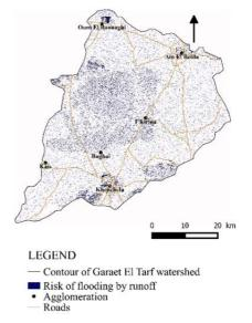
Fig. 8. Card of risk flooding by runoff at Gareat El Taref catchment; source: own elaboration
