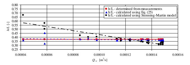
Fig. 7. Vertical pipe submergence ratio (h/L) for the delivery head H = 1.35 m
