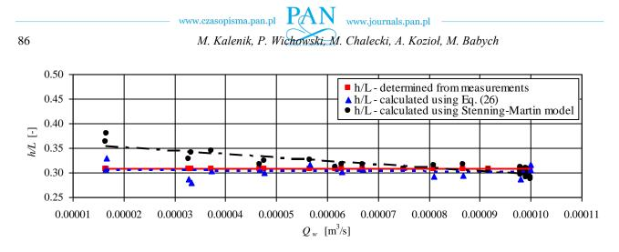
Fig. 8. Vertical pipe submergence ratio (h/L) for the delivery head H = 1.80 m
