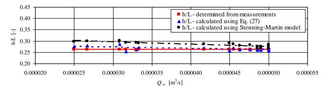
Fig. 9. Vertical pipe submergence ratio (h/L) for the delivery head H = 2.25 m
