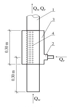
**Fig. 2.** Construction of the air-water mixer: 1 - transparent vertical pipe, 2 - steel end joining the elastic air supplying pipe, 3 - mixing chamber, 4 – holes.
