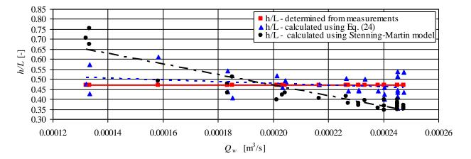
Fig. 6. Vertical pipe submergence ratio (h/L) for the delivery head H = 0.90 m
