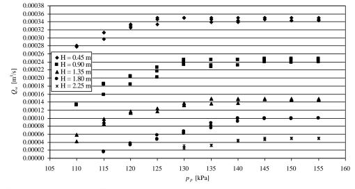
**Fig. 4.** Water flow rate  $(Q_w)$  in the air lift pump vs. air pressure  $(p_p)$  and water delivery height (H)
