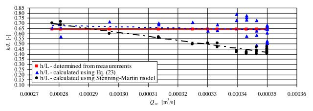
Fig. 5. Vertical pipe submergence ratio (h/L) for the delivery head H = 0.45 m
