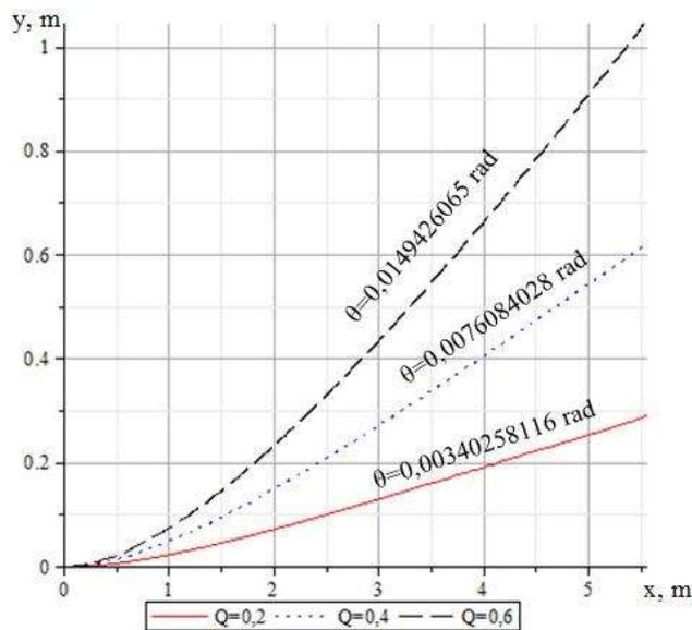
**Fig.4.** Motion trajectory of the center of mass for different values of  $Q_0$  and corresponding values of  $\theta$  (for the model with wheel track taken into account)
