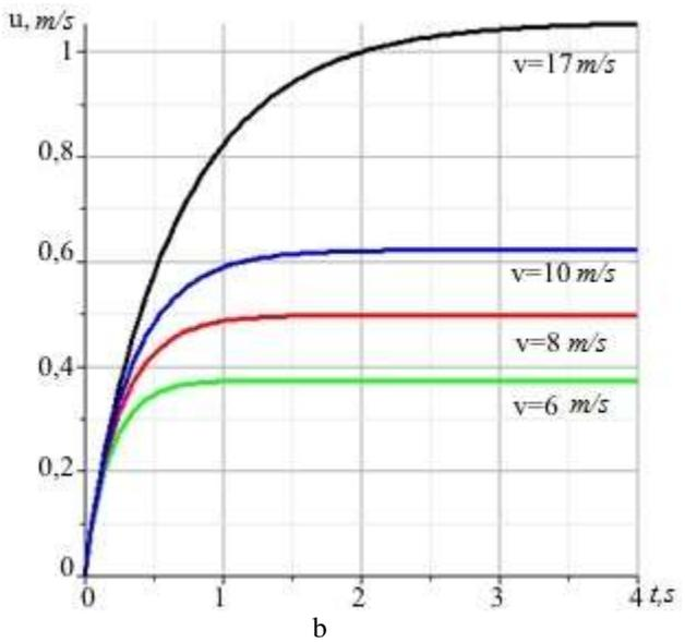
Fig. 2. Integral curves  $\omega(t)$  and  $u(t)$  for different values of speed
