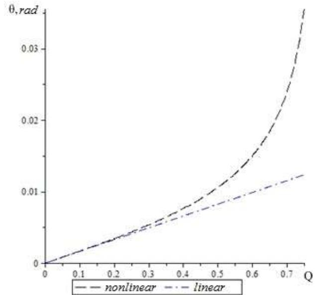
**Fig.1.** The external lateral force compensation chart.  $\theta=f(Q)$  acc. to linear and nonlinear drift hypothesis
