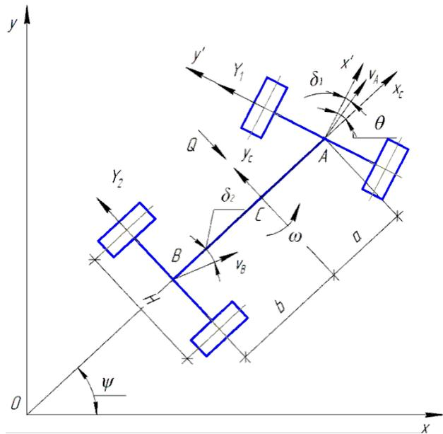
Fig.3. Car model with the “rigid” steering wheel module
