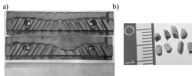
Fig. 1. Excessively worn lining surface (a) resulting in increased percentage share of large-size particle fraction with excessive size (b), unacceptable for the chipboard production process
