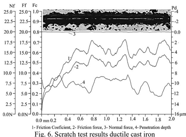
Fig. 6. Scratch test results ductile cast iron
