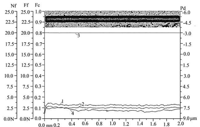
Fig. 5. Scratch test results for WCCoCr coating
