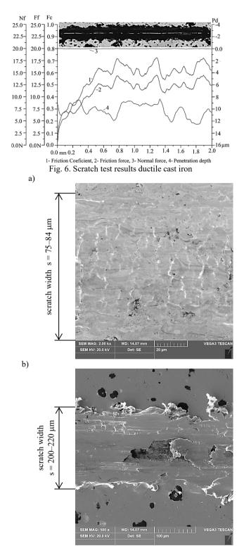
Fig. 7. A view of surface of scratches made on (a) WCCoCr coating and (b) on ductile cast iron substrate. Non-etched sections
