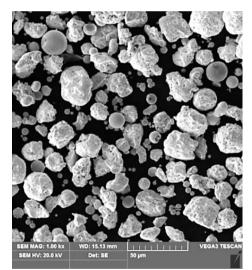
Fig. 3. WCCoCr 86104 powder particles
