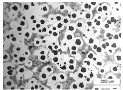
Fig. 2. Microstructure of substrate material. Graphite, ferrite and pearlite. Section etched with Nital. Magnification ×100
