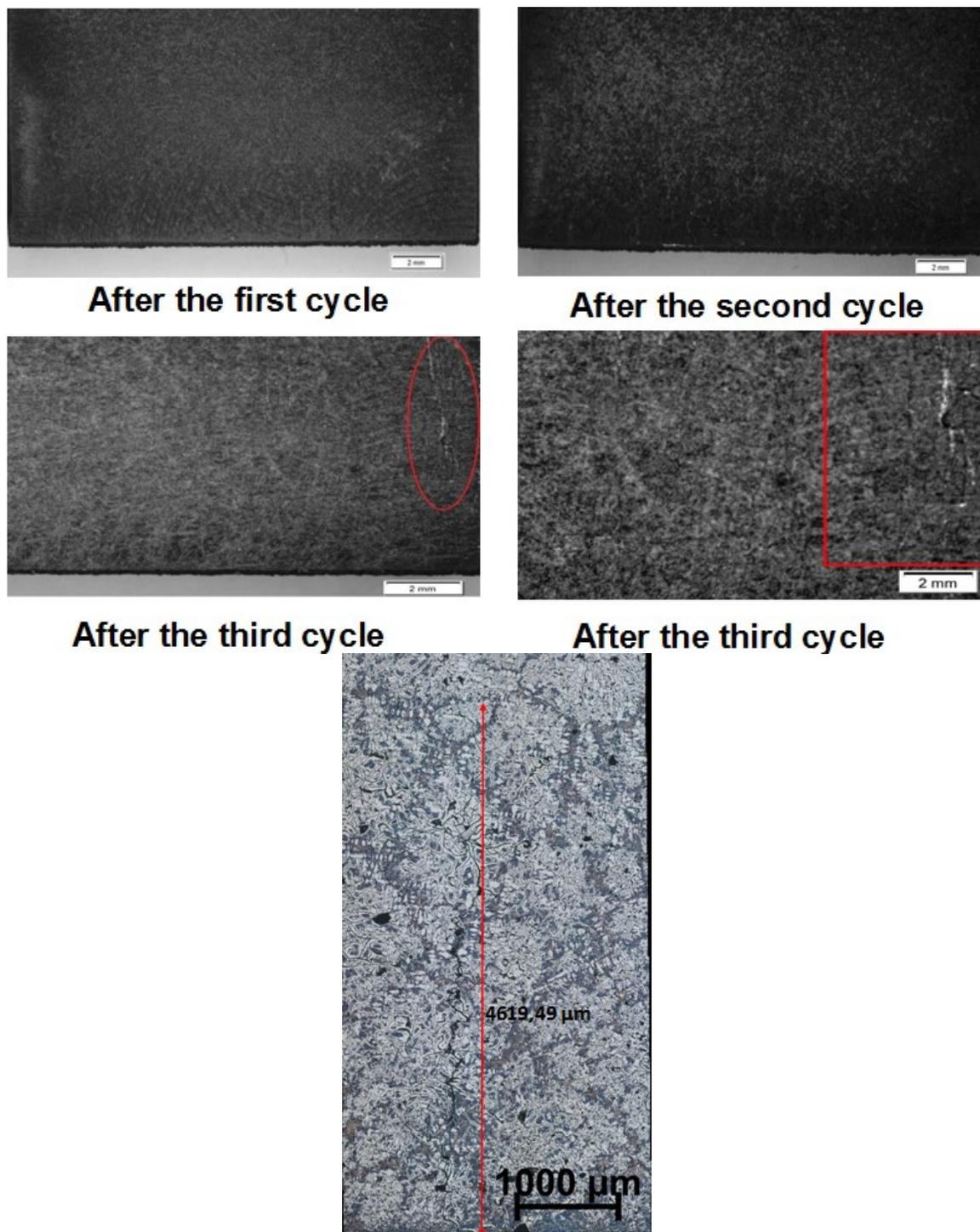
Fig. 9. Macroscopic view of samples after cycles of test and view of microstructure with marked length of cracks- Grey cast iron
