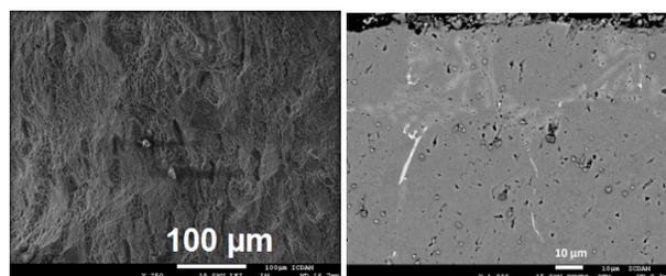
Fig. 2, 3. Inclusions in structure observed by electron microscopy
