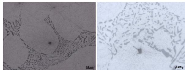
Fig. 4, 5. Inclusions in primary  $\alpha(\text{Al})$  phase observed by light microscopy
