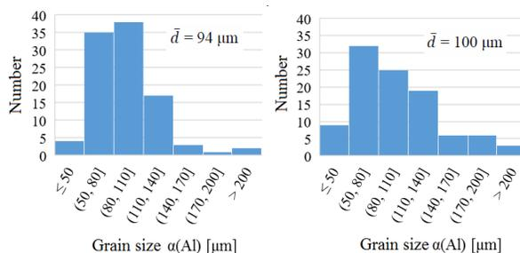
Fig. 23, 24. Average grain size – no inoculation (left), 0,05 % AlTi5B1 (right)
