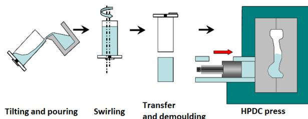
Fig. 1. SEED rheocasting method principle – phases [2]
