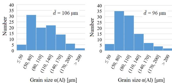
Fig. 25, 26. Average grain size - 0,1 % AlTi5B1 (right), 0,15 % AlTi5B1 (right)
