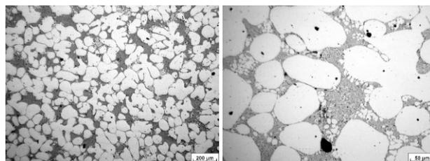
Fig. 18, 19. Structure inoculated by 0,15 % AlTi5B1
