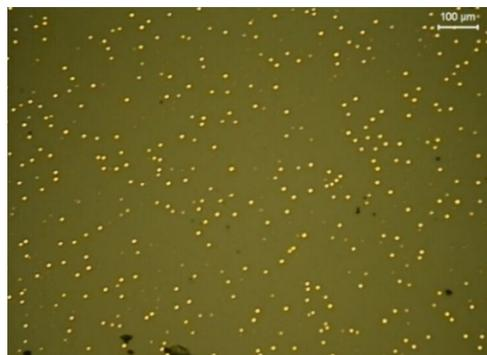
Fig. 6. Agglomeration and coagulation of the droplets in slag
