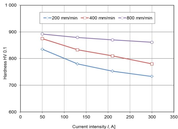
Fig. 7. The effect of the electric arc current intensity and the speed of scanning with electric arc on hardness of remeltings made on nodular cast-iron plate casting
