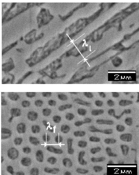
Fig. 1. Determination of structural parameter  $\lambda$  in lamellar and fibrous cementite eutectic
