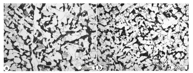
Fig. 4. Microstructure of as-cast steel, a) without REMs, b) with the REM additive, LM; nital etched
