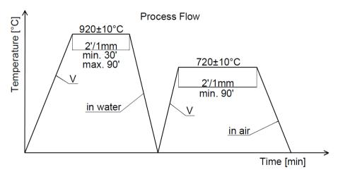
Fig. 2. Process flow of heat treatment
