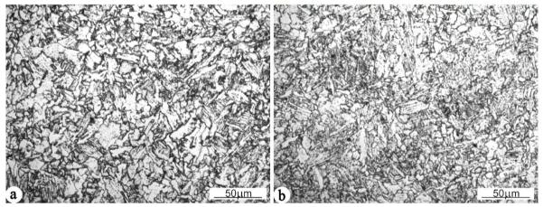
Fig. 5. Microstructure of heat-treated cast steel, a) without REMs, b) with the REM additive, LM; nital etched
