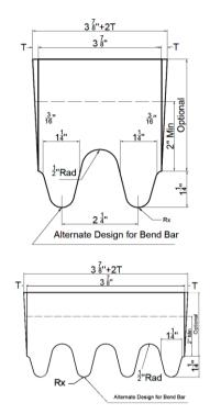
Fig. 1. Scheme of test ingots in compliance with ASTM A370-77
