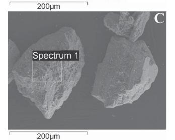
**Fig. 12.** Representative sands from the YD profiles un-affected by theorized cosmic airburst; A – Subangular to angular grains of the Cox horizon in the G1 paleosol; B – Angular hornblende; C – Angular pyroxene, possibly augite.
