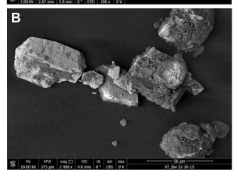
**Fig. 5.** A – General frame of grains in G11-Bw, some welded together and all of silt and very fine sand grain size; B – General frame of grains in V7-Bw, ranging from silt to near middle sand grade size and welded grains, with one large spherule of very fine sand. These grains are typical of the population of minerals recovered from all mid-LG sites in the upper Po and Guil catchments.
