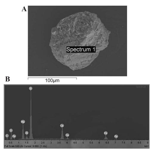
Fig. 10. A – Spherule-formed grain of variable composition with welded fragments in V9-Bw (see Mahaney *et al.*, 2013d for section details); B - EDS spot analysis of one grain, amid the collective assemblage of welded grains, highlights a terrestrial composition of Si:Al = 9:1, with near equal ratios of Ca:Mg, with low Fe and lower C, possibly augite but with low Al.
