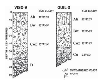
**Fig. 2.** Typical profiles in the upper Guil (GUIL-3) and upper Po (VISO-9) catchments. Some profiles have sufficient matrix sediment to qualify as Cu horizons; others are an open network of coarse clastic sediment termed 'D'. Morphogenetic details on these and other paleosols in the Guil-Po corridor are in Mahaney and Keiser (2013) and Mahaney *et al.* (2016a).
