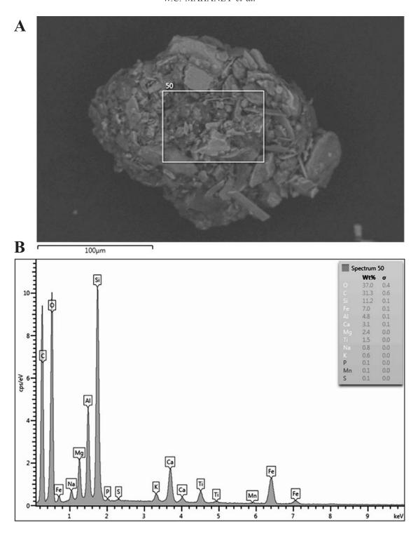
**Fig. 6.** A – Airburst grain from G11-Bw composed of welded minerals of variable composition, all sourced from local metabasalt and with high carbon content; B – The sample was analyzed without conductive coating so the carbon content is real.
