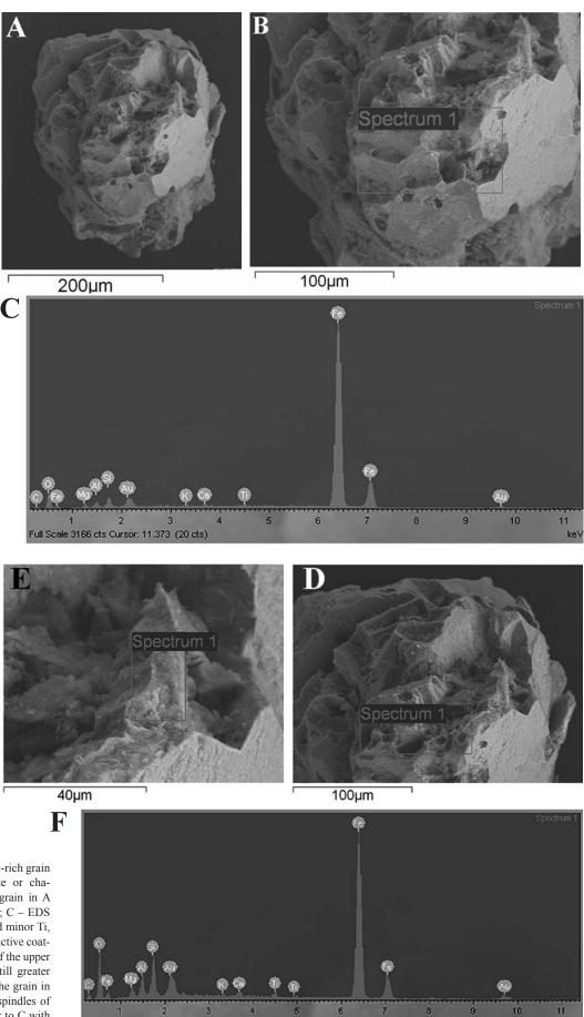
Fig. 11. A – Shock-melted Fe-rich grain in G3-Ah, possibly magnetite or chamosite; B – Enlargement of grain in A showing area of EDS analysis; C – EDS analysis highlights high Fe and minor Ti, Ca, K, Mg. The Au is the conductive coating; D – Greater enlargement of the upper part of the grain in A; E – Still greater enlargement of upper part of the grain in A showing details of welded spindles of Fe; F – EDS chemistry similar to C with slightly higher Si and Al.
