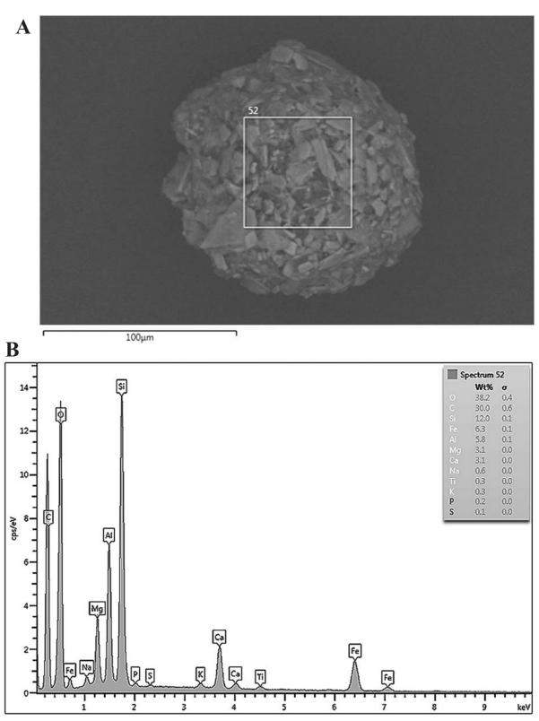
Fig. 7. A – Spherule from G11-Bw with near elliptical form; B – EDS indicates a similar composition to the compacted grains in Fig. 6.
