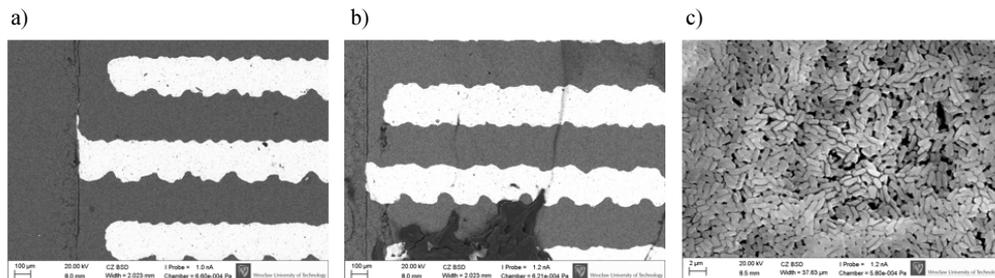
Fig. 4. SEM images of *P. aeruginosa* biofilm on the surfaces of LTCC sensors: a clean reference (a); after 16 h of incubation (b) and focused on a biofilm structure (d).
