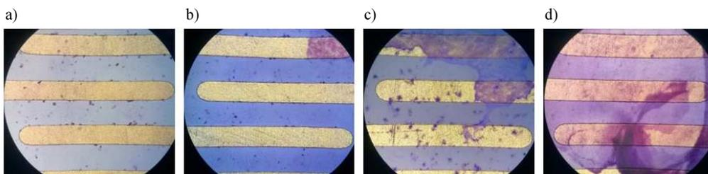
Fig. 3. Optical microscopy images (magnitude 40 x) of *P. aeruginosa* biofilm stained with a crystal violet on the surfaces of PCB sensors after: 1 hour (a); 4 hours (b); 16 hours (c) and 24 hours of incubation (d).
