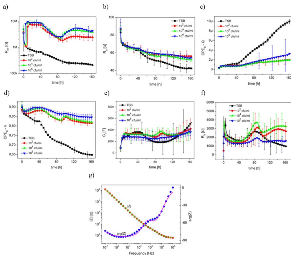
Fig. 6. Changes of mean value (points) and standard deviation (error bars) of EEC parameters in time during incubation:  $R_{CT}$  (a);  $R_S$  (b);  $CPE_B-Q$  (c);  $CPE_B-n$  (d);  $C_I$  (e);  $R_B$  (f); and examples of measured (dots) and fitted (lines) impedance spectra for  $10^2$  cfu/ml at 36th hour (g).
