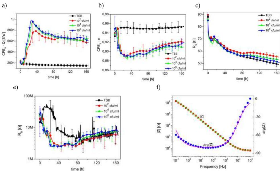
Fig. 7. Changes of mean value (points) and standard deviation (error bars) of EEC parameters in time during incubation:  $CPE_B-Q$  (a);  $CPE_B-n$  (b);  $R_S$  (c);  $R_B$  (d); and examples of measured (dots) and fitted (lines) impedance spectra for  $10^2$  cfu/ml at 36th hour (e).
