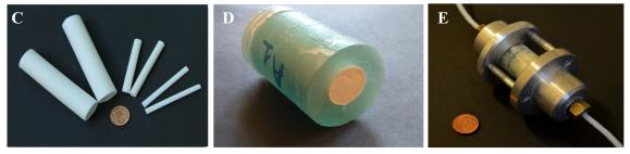
Fig. 1. SEM image of monolith structure applied as GMR- (A) and MMR- (B) type of microreactor, images of monoliths used in GMRs (C), a single monolith embedded into polymeric shell (D), image of a typical GMR (E)
