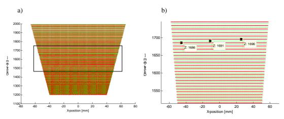
Fig. 2. Iso-disparities obtained by simulation before and after applying the dither signal. Red lines come from the primary and green lines were obtained after the dither signal. b) Zoomed-in area (inside the box) of a).
