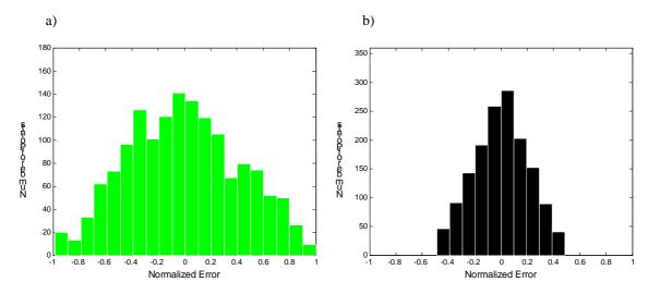
Fig. 5. Histograms of the normalized depth reconstruction error a) for the direct triangular method and b) after applying the dithering algorithm.
