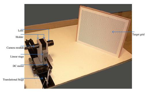
Fig. 6. A side view of the camera prototype showing its components and the experiment setup.
