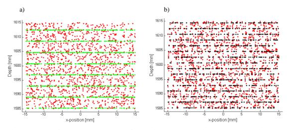
Fig. 4. Top view of the depth reconstruction of the original target points (in red). The green points represent the reconstructed points by the direct method; b) describes the reconstructed points by the dithering algorithm as black points.
