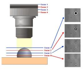
Fig. 3. Principle of vertical scanning in interferometry.
