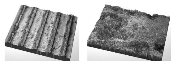
Fig. 4. Brake drum (left) and lining (right), 0 kilometres of covered distance.
