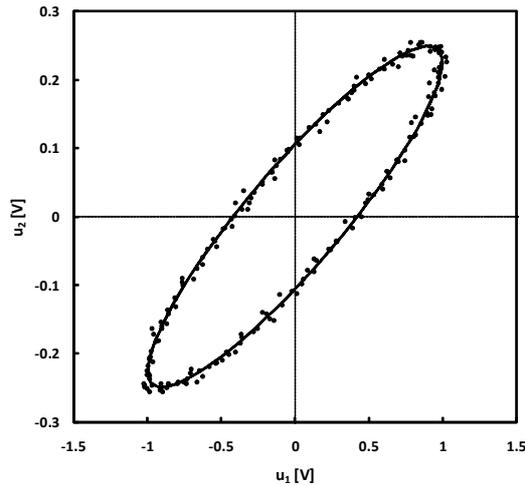
Fig. 1. Ellipse fit of two sinewaves with  $D_1 = 1$  V,  $D_2 = 0.25$  V,  $f = 1$  kHz,  $\Delta\phi = 25^\circ$  and  $N = 200$ . The dots represent the sampled data and the line represents the fitted ellipse.
