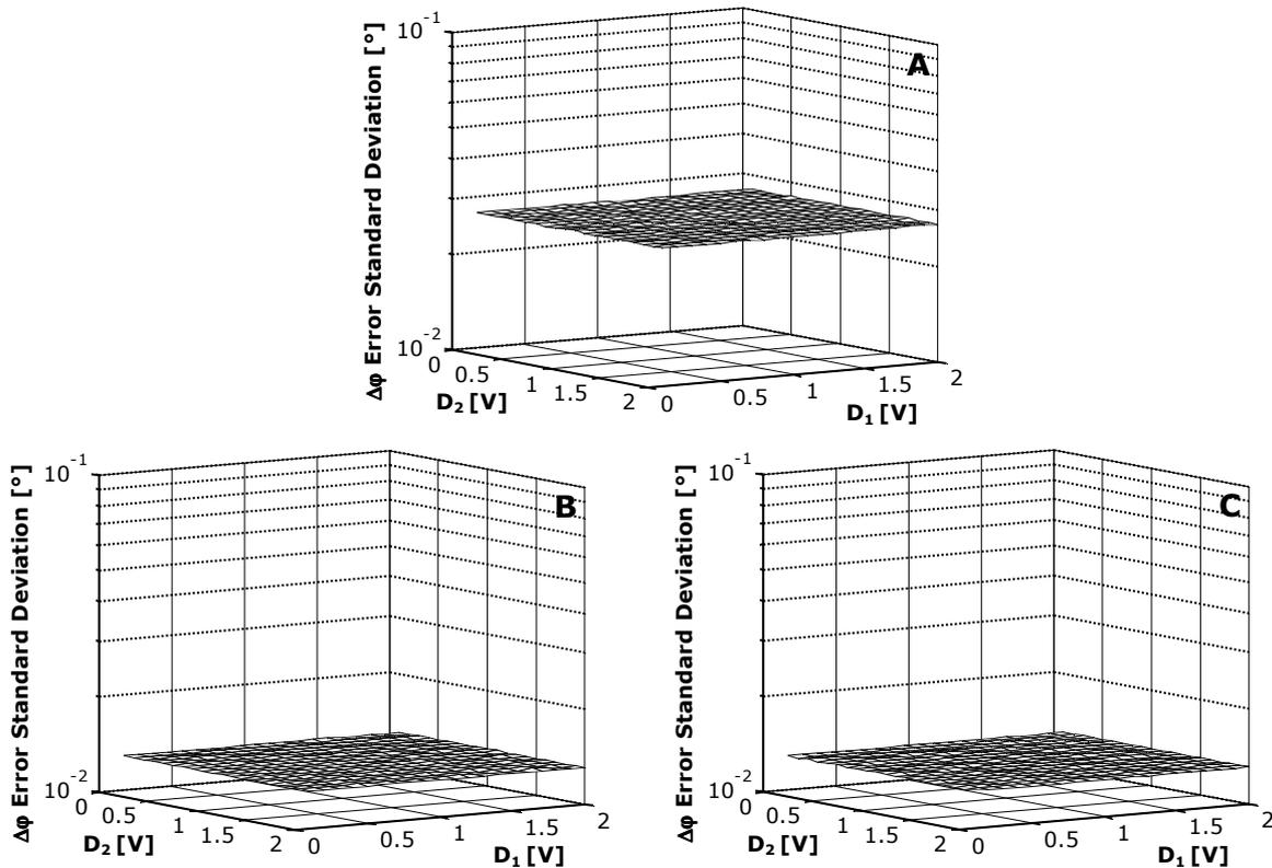
Fig. 10. Standard deviation of the estimated phase error for the ellipse fit (A), seven parameter sine fit (B) and spectral sinc fit (C) as a function of the two signal amplitudes for  $SNR_1=40$  dB and  $SNR_2=80$  dB.
