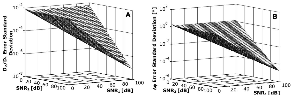
Fig. 7. Standard deviation of the amplitude ratio (A) and phase difference error (B) for the spectral sinc fit algorithm as a function of the two signal to noise ratios for  $D_1=1$  V and  $D_2=0.25$  V.
