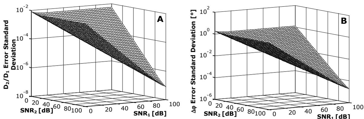
Fig. 6. Standard deviation of the amplitude ratio (A) and phase difference error (B) for the seven parameter sine fit algorithm as a function of the two signal to noise ratios for  $D_1=1$  V and  $D_2=0.25$  V.
