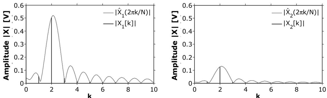
Fig. 3. Spectral sinc fit: positive frequencies of the two-sided amplitude spectrums of two sinewaves ( $D_1 = 1$  V,  $D_2 = 0.25$  V,  $f = 1$  kHz,  $\Delta\phi = 25^\circ$  and  $N = 200$ ) and the fitted spectrum.
