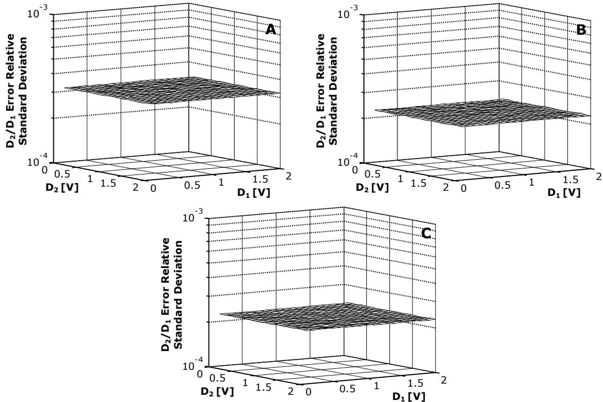
Fig. 9. Relative standard deviation of the amplitude ratio for the ellipse fit (A), seven parameter sine fit (B) and spectral sinc it (C) as a function of the two signal amplitudes for  $SNR_1=40$  dB and  $SNR_2=80$  dB.
