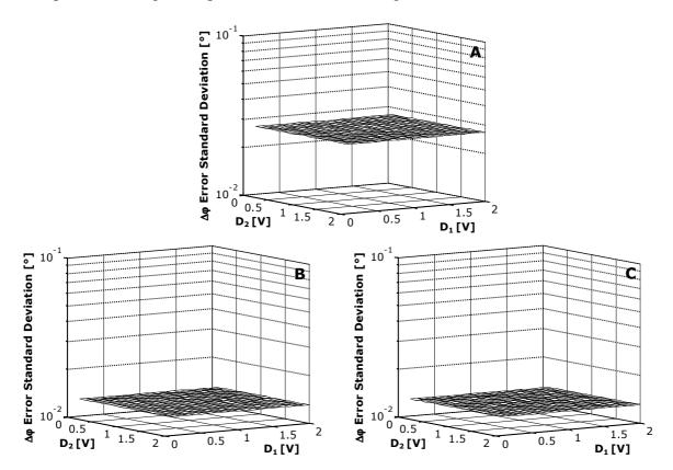
Fig. 10. Standard deviation of the estimated phase error for the ellipse fit (A), seven parameter sine fit (B) and spectral sinc fit (C) as a function of the two signal amplitudes for SNR<sub>1</sub>=40 dB and SNR<sub>2</sub>=80 dB.
