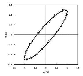
Fig. 1. Ellipse fit of two sinewaves with  $D_1 = 1$  V,  $D_2 = 0.25$  V, f = 1 kHz,  $\Delta \varphi = 25^\circ$  and N = 200. The dots represent the sampled data and the line represents the fitted ellipse.
