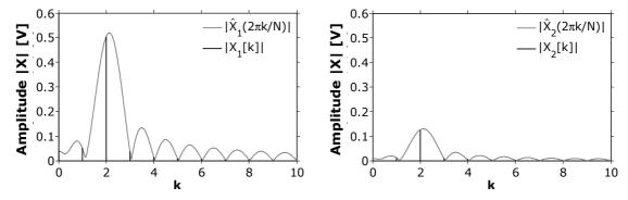
Fig. 3. Spectral sinc fit: positive frequencies of the two-sided amplitude spectrums of two sinewaves  $(D_1 = 1 \text{ V}, D_2 = 0.25 \text{ V}, f = 1 \text{ kHz}, \Delta \phi = 25^{\circ} \text{ and } N = 200)$  and the fitted spectrum.
