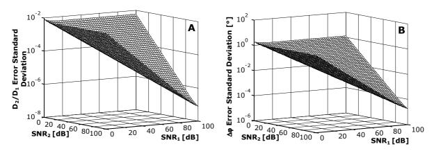
Fig. 7. Standard deviation of the amplitude ratio (A) and phase difference error (B) for the spectral sinc fit algorithm as a function of the two signal to noise ratios for  $D_1$ =1 V and  $D_2$ =0.25 V.
