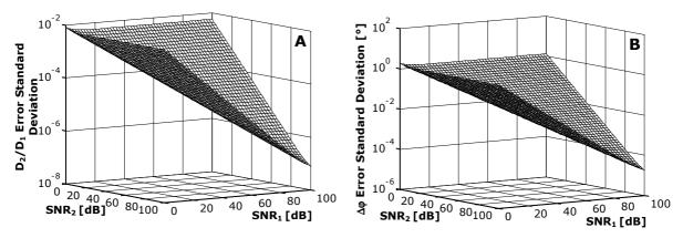
Fig. 6. Standard deviation of the amplitude ratio (A) and phase difference error (B) for the seven parameter sine fit algorithm as a function of the two signal to noise ratios for  $D_1$ =1 V and  $D_2$ =0.25 V.
