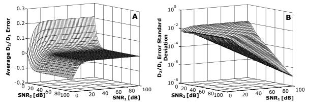
Fig. 4. Average amplitude ratio error (A) and corresponding standard deviation (B) for the ellipse fit algorithm as a function of the two signal to noise ratios for  $D_1$ =1 V and  $D_2$ =0.25 V.
