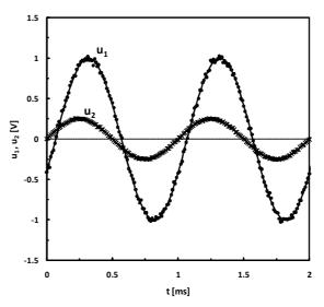
Fig. 2. Seven-parameter sine fit of two sinewaves with  $D_1 = 1 \text{ V}$ ,  $D_2 = 0.25 \text{ V}$ , f = 1 kHz,  $\Delta \phi = 25^{\circ}$  and N = 200. The dots represent the  $u_1$  sampled data, the crosses represent the  $u_2$  sampled data and the lines represent the reconstructed sinewaves.
