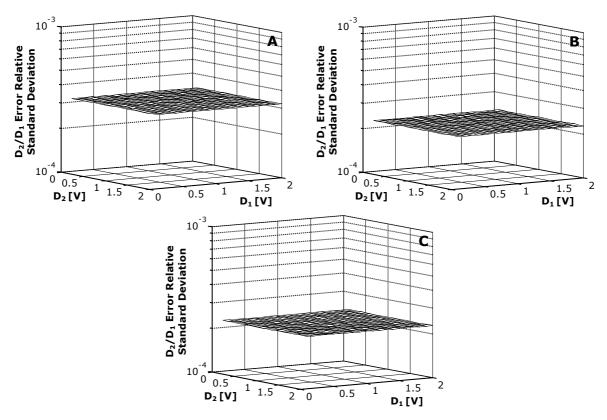
Fig. 9. Relative standard deviation of the amplitude ratio for the ellipse fit (A), seven parameter sine fit (B) and spectral sine it (C) as a function of the two signal amplitudes for  $SNR_1=40$  dB and  $SNR_2=80$  dB.
