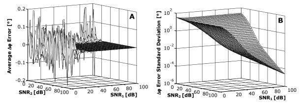
Fig. 5. Average phase difference error (A) and corresponding standard deviation (B) for the ellipse fit algorithm as a function of the two signal to noise ratios for  $D_1$ =1 V and  $D_2$ =0.25 V.
