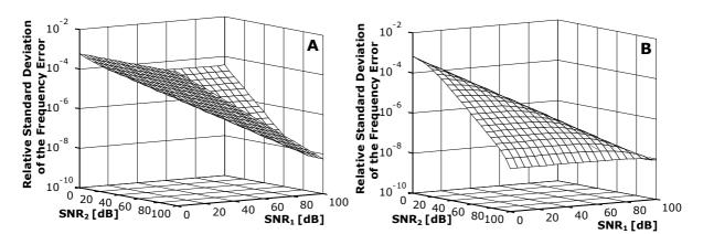
Fig. 8. Relative standard deviation of the estimated frequency error for the seven parameter sine fit algorithm (A) and for the spectral sine fit algorithm (B) as a function of the two signal to noise ratios for  $D_1$ =1 V and  $D_2$ =0.25 V.
