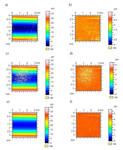
Fig. 5. Contour plots of a worn cylinder surface before (a, c, e) and after form removal (b, d, f) with non-measured points located in a valley region; NM ratio 4.31%(a, b), in a peak part; NM ratio 14.4% (c, d) and with their smallest number; NM ratio 0.102% (e, f).
