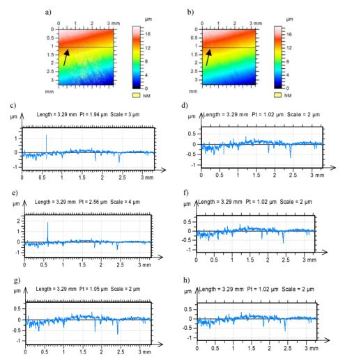
Fig.7. Contour plots (a, b), extracted profiles before correction – filling in (c, d), after correction of the whole surface (e, f) and after profile correction (g, h); NM ratio 6.68% (a, c, e, g) and 0.079% (b, d, f, h).
