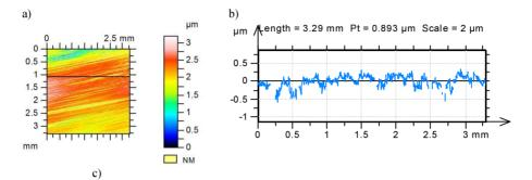
$Sq = 0.387 \ \mu\text{m}; Sp = 1.13 \ \mu\text{m}; Sv = 2.03 \ \mu\text{m}; Ssk = -0.76; Smr = 49.1\%$
