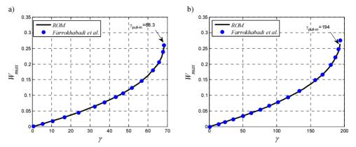
Fig. 3. Variations of the static deflection vs the Casimir force for (a) SSA approximation (k = 5) and (b) LSA approximation (k = 100), and for  $\alpha_k = 1$ ,  $\alpha_k, \kappa_1, \sigma_2, \alpha_k, \kappa_2 = 0$ .
