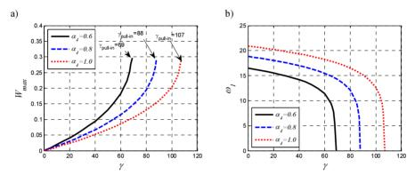
Fig. 10. Variations of (a) the static deflection and (b) the natural frequency vs the Casimir force for SSA approximation and  $\sigma_2 = 2$ .
