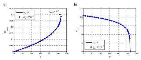
Fig. 5. Variations of (a) the static deflection and (b) the natural frequency vs the Casimir force for SSA approximation and k = 10,  $\alpha_4 = 1$ ,  $\sigma_2 = 2$
