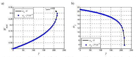
Fig. 4. Variations of (a) the static deflection and (b) the natural frequency vs the Casimir force for LSA approximation and k = 100,  $\alpha_4 = 1$ ,  $\sigma_2 = 2$ .
