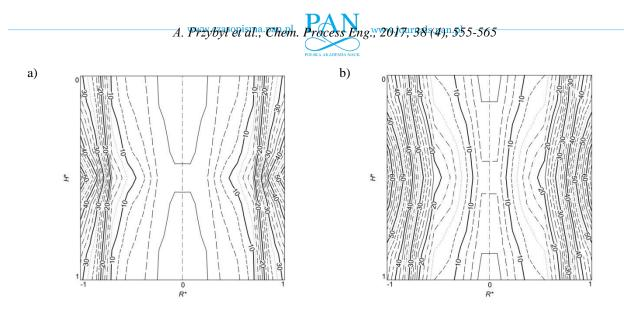
Fig. 4. A typical example of magnetic field patterns: a) f = 10 Hz, b) f = 50 Hz
