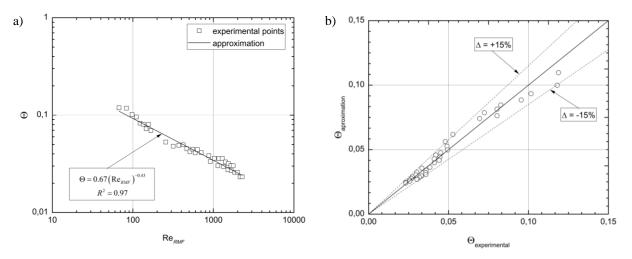
Fig. 7. The dependence of  $\Theta = f(\text{Re}_{RMF})$  (a) and comparison of the experimental and calculated values or the dimensionless mixing time number (b)
