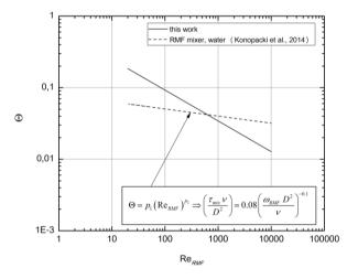
Fig. 8. A comparison of the dimensionless mixing time for systems enhanced by RMF and the RMF mixer (Konopacki et al., 2014)
