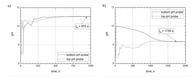
Fig. 3. Typical example of pH transient processes (pH changes during mixing time investigation) at f = 30 Hz for: a) H-S medium, b) distilled water
