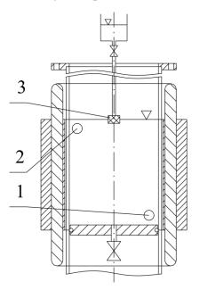
Fig. 2. Localization of the pH electrodes (1, 2) and the injection point (3)
