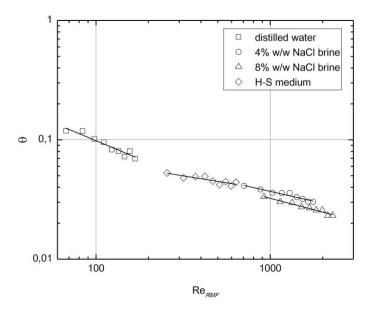
Fig. 6. The dependence of  $\Theta = f(\text{Re}_{RMF})$  for the analyzed liquids
