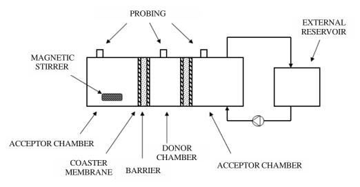
Fig. 4. SU4: Sequential Unit system imitating drug-eluting stent placed within the blood vessel
