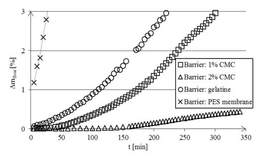
Fig. 7. The relative mass increase of substance in SU2 system (with flow) in acceptor chamber; diffusion through different mass transfer barriers, solution of Cochineal Red A (1%)
