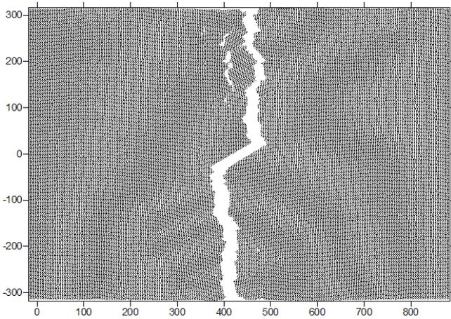
Fig. 4. Deformation at extension 4.1%
