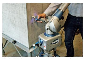
Fig. 6. Tank during measurements and visible reference points placed on a supporting steel frame
