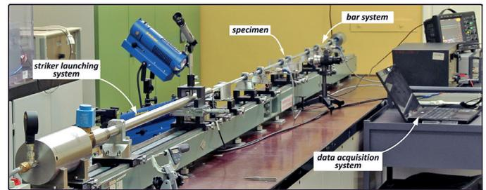
Fig. 1. View of the arrangement used for classical split Hopkinson compression bar
