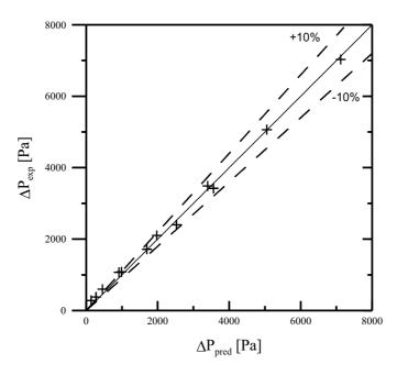
Figure 2: Comparison of single-phase pressure drop experimental data for the R134a with the predicted Darcy-Weisbach correlation.
