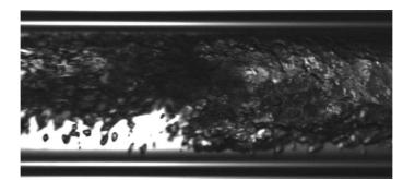
Figure 9: Experimentally obtained intermittent adiabatic flow of R134a for  $G = 400 \text{ kg/m}^2 \text{s}$  with  $\dot{q} = 9.5 \text{ kW/m}^2$ , point B on flow pattern map.
