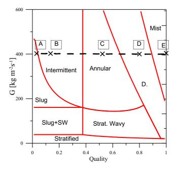
Figure 7: Flow pattern map evaluated for R134a at  $T_{sat} = 19.4$  °C in a 5 mm internal diameter tube for  $\dot{q} = 35$  kW/m<sup>2</sup> using G = 400 kg/m<sup>2</sup>s to calculate the void fractions.
