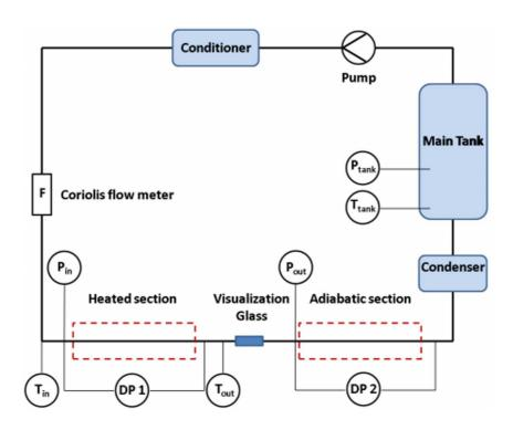
Figure 1: Schematic diagram of test facility:  $P_{tank}$  – pressure in the tank,  $P_{out}$  – pressure at the outlet of heated section,  $T_{out}$  – temperature at the outlet of the heated section,  $T_{in}$  – temperature at the inlet of the heated section,  $T_{tank}$  – temperature in the tank, DP1 – pressure drop at the heated section, DP2 – pressure drop at the adiabatic section.
