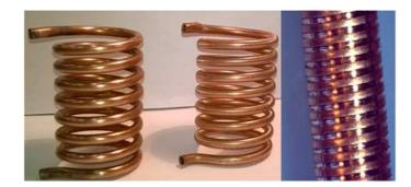
Figure 3: Obtained construction of helical coils: at the left side – coil made from smooth copper pipe, in the middle - coil with modified surface, at the right side photo of modified surface.
