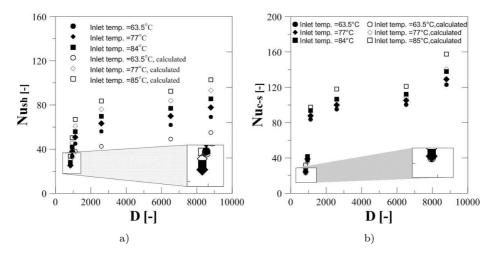
Figure 10: Variation of Nusselt number with Dean number for different fluid inlet temperature in case of unmodified surface: a) for shell side, b) for coil side.
