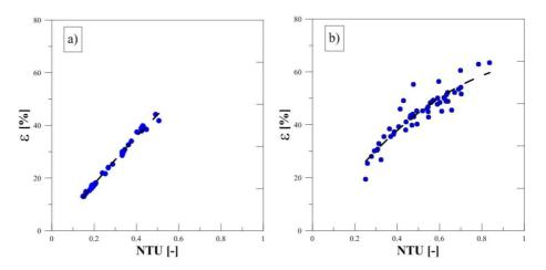
Figure 12: Experimentally obtained modified heat exchanger effectiveness in function of NTU for: a) parallel flow configuration, b) counter-flow configuration.
