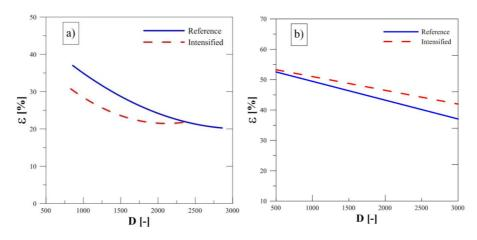
Figure 13: Effectiveness of helical coils heat exchanger, as a function of the Dean number (D): a) parallel flow configuration, b) counter-flow configuration.
