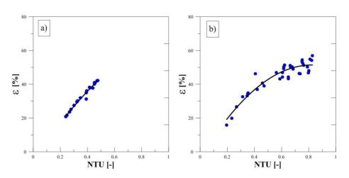
Figure 11: Experimentally obtained reference heat exchanger effectiveness in function of NTU for: a) parallel flow configuration, b) counter-flow configuration.
