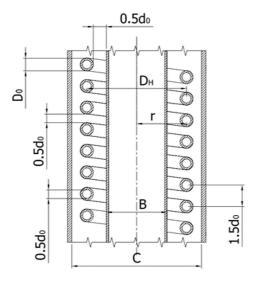
Figure 2: Geometrical assumptions for designed helical heat exchanger.
