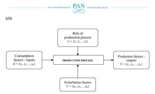
Fig. 4. Principle schema of the production process
