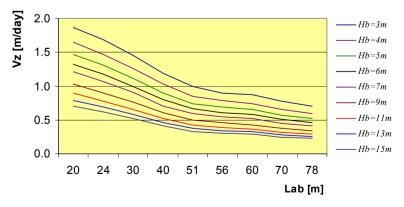
Fig. 13. Variation of the daily face advancement speed  $V_z = f(l_{ab})$ , in function of the coal face length, for  $N_{shift} = 6$  workers
