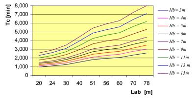
Fig. 11. Variation of the coal face cycle  $T_c = f(l_{ab})$ , in function of the coal face length, for  $N_{shift} = 6$  workers
