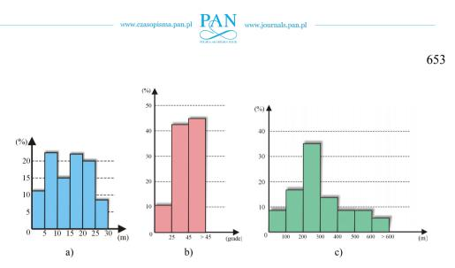
Fig. 1. Histograms of the main geometrical characteristics of the coal seam no. 3 – Jiu Valley coal basin: a) thicknesses; b) dips; c) block lengths (Onica, 1995)
