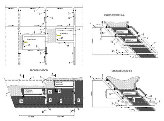
Fig. 5. Longwall faces top coal caving mining method, in horizontal slices, applied at the coal seam no. 3, for the dip of  $\geq$  45°
