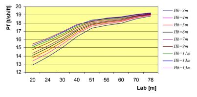
Fig. 16. Variation of the workforce productivity  $P_f = f(l_{ab})$ , in function of the coal face length, for  $N_{shift} = 6$  workers
