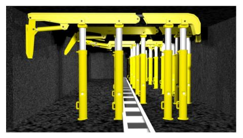
Fig. 6. Frame powered supports type GEROM GP 250/12
