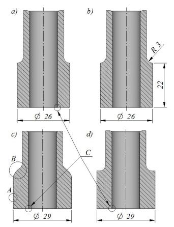
Fig. 2. Forgings in the final stage of extrusion with a moving sleeve; denoted in accordance with Table 1: a) Case 1, b) Case 2, c) Case 3, d) Case 4.
