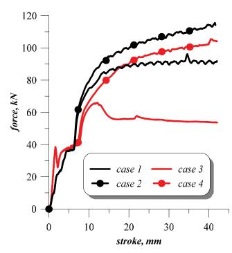
Fig. 5. Variations in punch-applied force versus its displacement for the investigated extrusion cases
