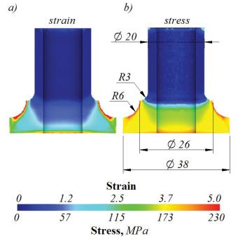
Fig. 6. Distributions of: a) effective strains, b) reduced stresses in the forging with a two-step flange
