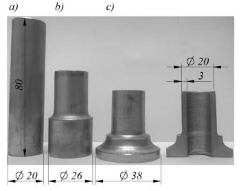
Fig. 7. Forgings produced in experimental tests: a) billet, b) one-step flange, c) two-step flange
