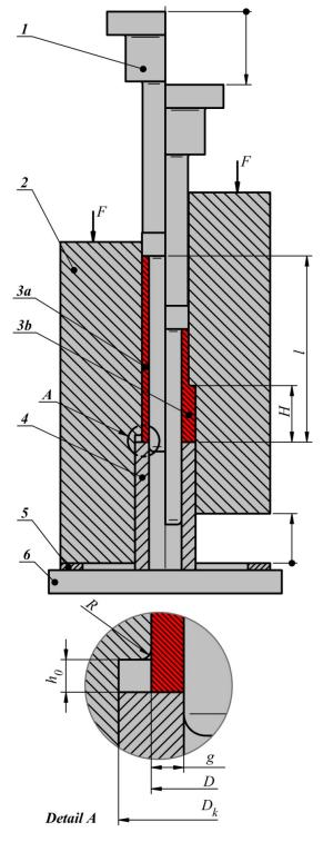
Fig. 1. Schematic design of a process for forming flanges by extrusion with a movable sleeve; 1 - punch, 2 - moving sleeve, 3a - billet, 3b - forging, 4 - fixed sleeve, 5 - distance plate, 6 - base
