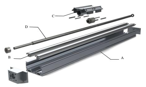
Fig. 6. View of a compact linear module. A – aluminium housing (body 1), B – a set of rails, C – table (body 2), D – ballscrew mechanism with bearings
