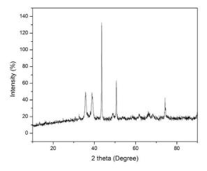
Fig. 1. XRD pattern of CuO nanoparticle
