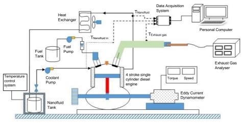
Fig. 3. Schematic diagram of experimental setup
