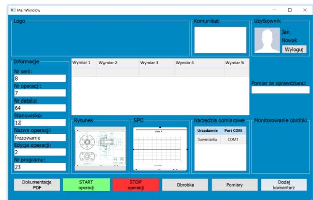
Fig. 5. The main window of operator panel – test version.
