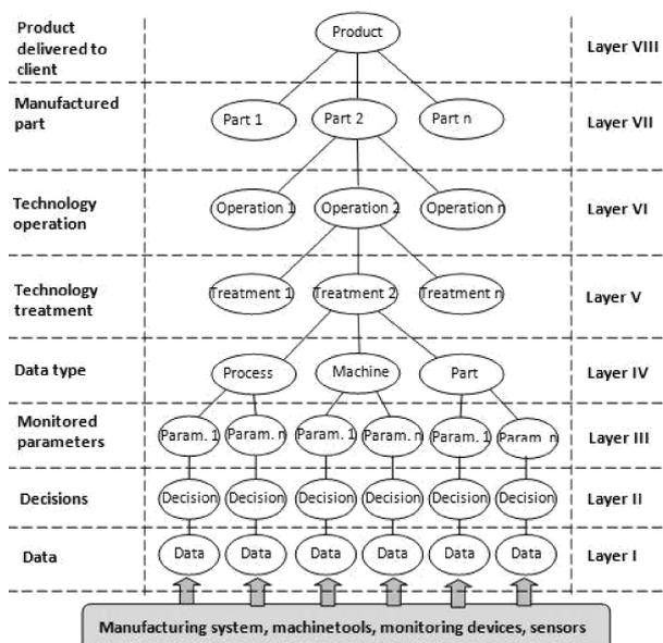
Fig. 8. Multilayer reference model of data integration for manufacturing process.
