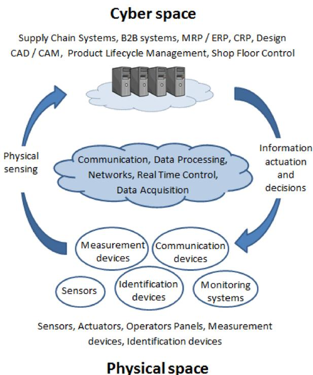
Fig. 9. Conception of the Cyber-Physical-Systems implementation in monitoring of discrete production process and integration of machine operators with Shop Floor Control.
