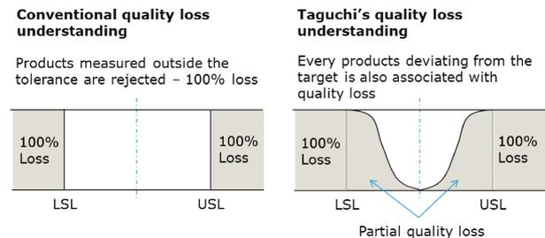
Fig. 3. Traditional and Taguchi loss function compared.
