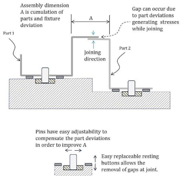
Fig. 10. A sheet metal welding fixture design needs maturation scope.
