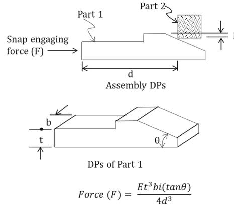
Fig. 7. Design parameters of the parts and assembly are highly interacting towards engaging force.
