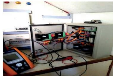
Fig. 11. PQ analyzer connected to extract the data
