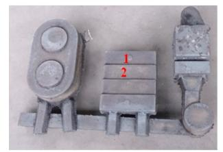
Fig. 1. Test castings with the gating system and reaction chamber
