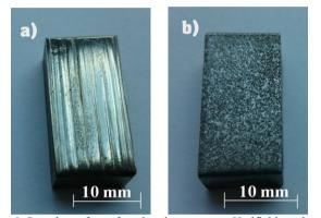
Fig. 6. Sample surface after abrasion test: cast Hadfield steel - a); tested cast steel with 2.0% Ti content - b)
