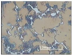
Fig. 2. As-cast microstructure of Hadfield steel with 1.4% Cr; austenitic matrix with numerous precipitates of alloyed cementite; nital etching [1]
