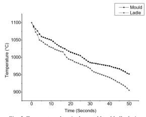
Fig. 5. Temperature drop in the mould and ladle during transportation
