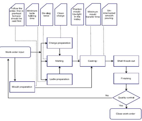
Fig. 9. Instruction card for casting operation at HF induction furnace
