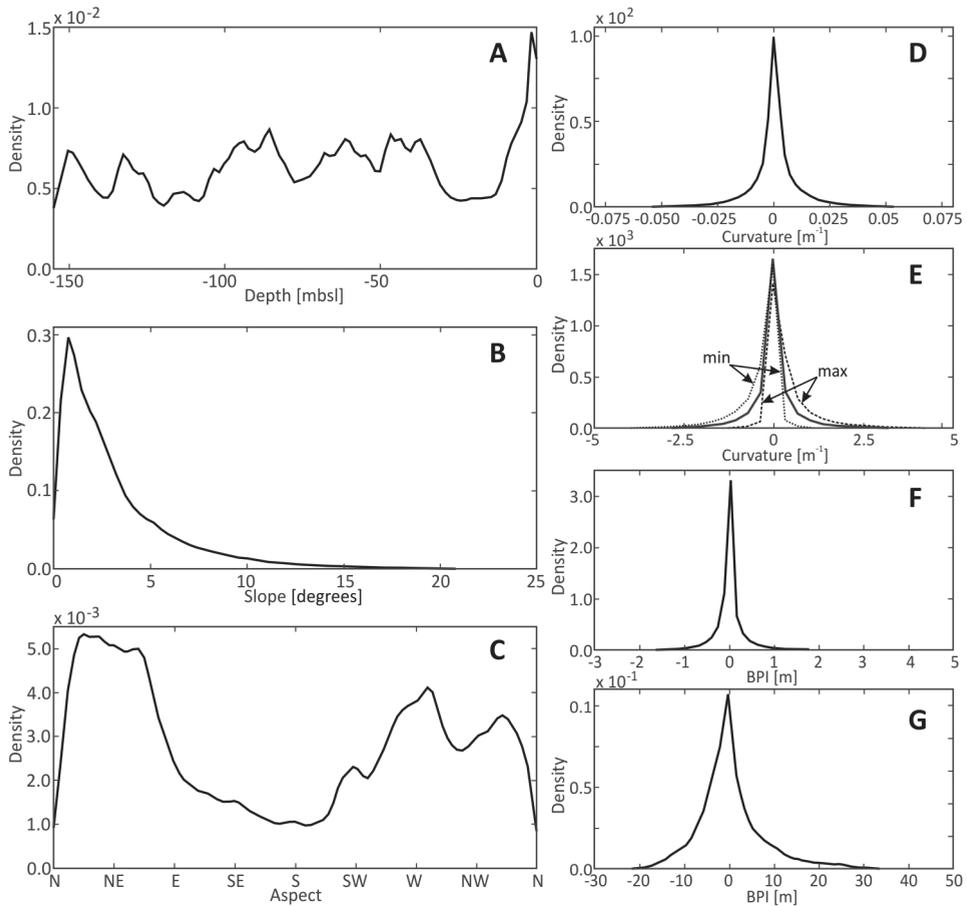
Fig. 5. Density distributions of (A) depth; (B) slope; (C) aspect; (D) contour curvature; (E) profile (black line), maximal (max) and minimal (min) curvatures; bathymetric position index (BPI) for (F)  $r_{min}=20$  m,  $r_{max}=50$  m and (G)  $r_{min}=200$  m,  $r_{max}=500$  m.
