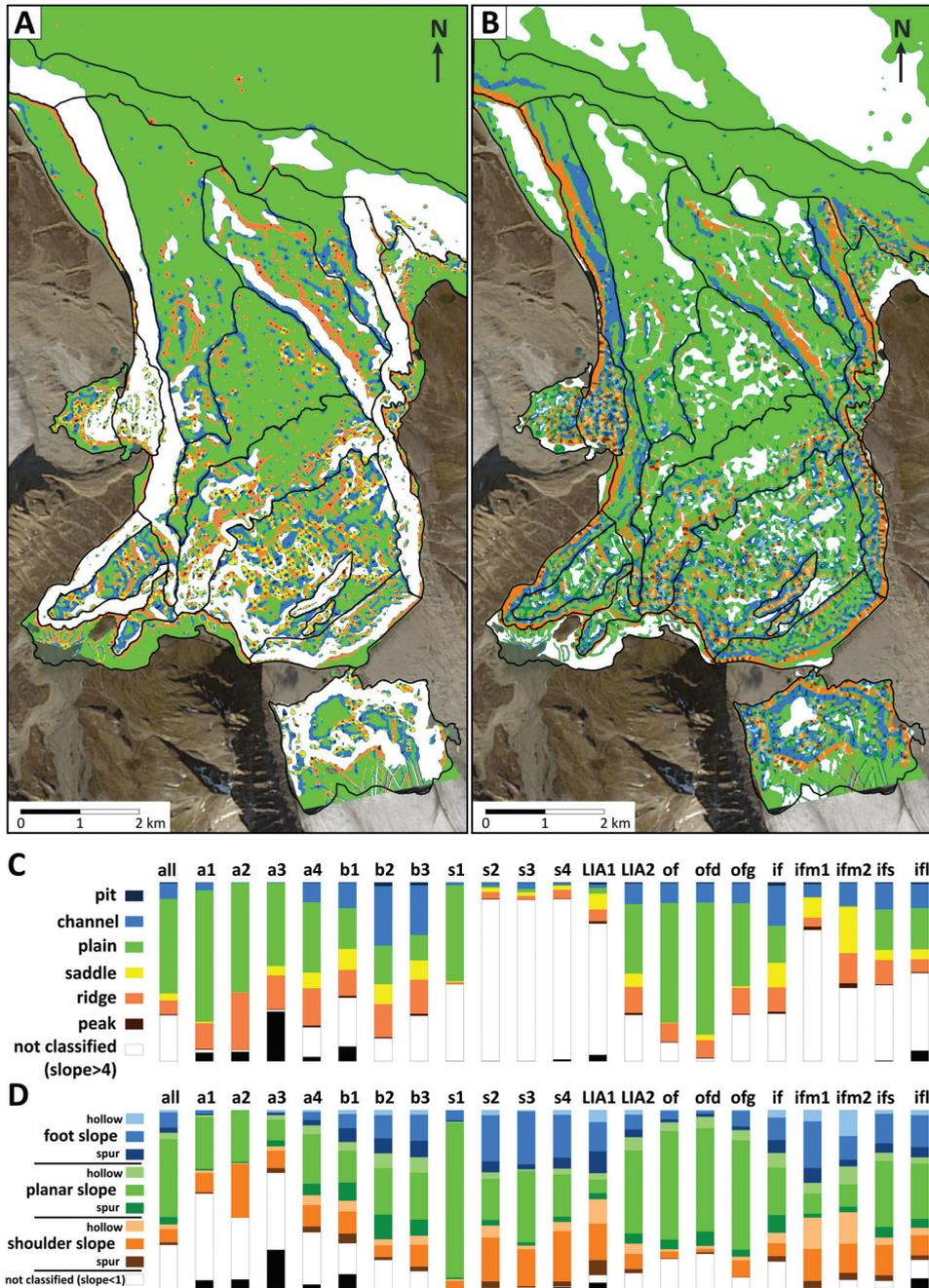
Fig. 6. Morphological parameters in study area (A, B) and their contribution in sets of landforms (C, D) base on maximal and minimal curvature – flat area elements (A, C), and contour and profile curvature – sloping elements (B, D). Sets of landforms described on Fig. 8.
