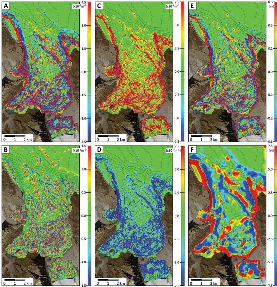
Fig. 4. Morphometric parameters: (A) profile curvature ( $prof_c$ ); (B) contour curvature ( $cont_c$ ); (C) maximal curvature ( $max_c$ ); (D) minimal curvature ( $min_c$ ); bathymetric position index (BPI) for (E)  $r_{min}=20$  m,  $r_{max}=50$  m, and (F)  $r_{min}=200$  m,  $r_{max}=500$  m.
