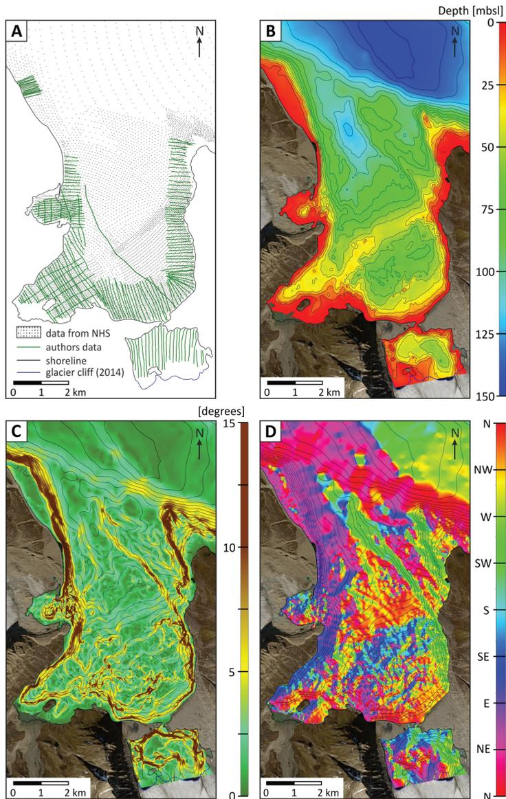
Fig. 2. (A) Measurements localisation; (B) Interpolated bathymetry; (C) slope; (D) aspect.
