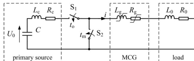
Fig. 3. The circuit model of the MCG.  $C, L_c, R_c$  are the capacity, inductance and resistance of the primary source, respectively, and  $L_g, R_g$  are the inductance and resistance of the MCG, respectively, and  $L_0, R_0$  are the inductance and resistance of the load, respectively
