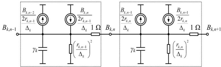
Fig. 5. Equivalent circuit of Equation (6) in node  $n$
