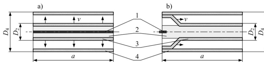
Fig. 2. Sketch of a coaxial MCG: a) the radial compression; b) the axial compression.  $D_4$  is the diameter of the external tube,  $D_2$  is the diameter of the internal tube: 1 – detonator, 2 – explosive material, 3 – internal tube, 4 – external tube
