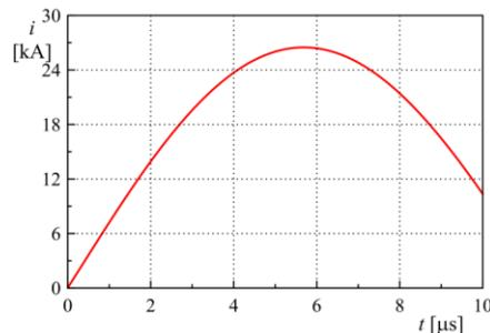
Fig. 6. Current profile in the MCG at constant resistance and inductance
