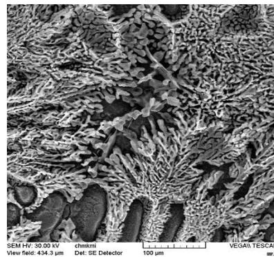
b) rod-shape of silicon, etch. HCl, REM
