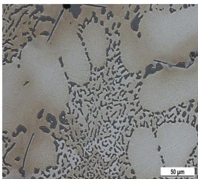
a) imperfectly rounded grains, etch. 0,5 % HF
