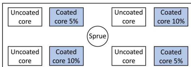
Fig. 2. Arrangement of experimental mould
