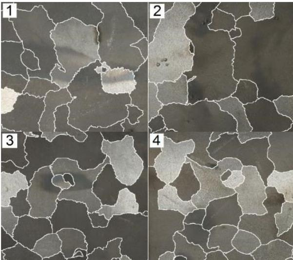
Fig. 5. Macrostructure comparison of specimens from sample 1: 1 – top inner (core), 2 – top outer (mould), 3 – bottom inner (core), 4 – bottom outer (mould)
