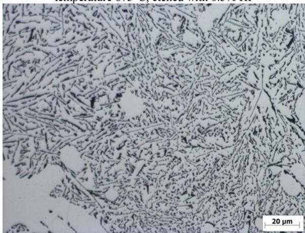
Fig. 10. Microstructure of samples, pressure 150 MPa, temperature 675°C, etched with 0.5% HF
