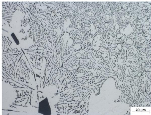
Fig. 6. Microstructure of samples, pressure 150 MPa, temperature 715°C, etched with 0.5% HF
