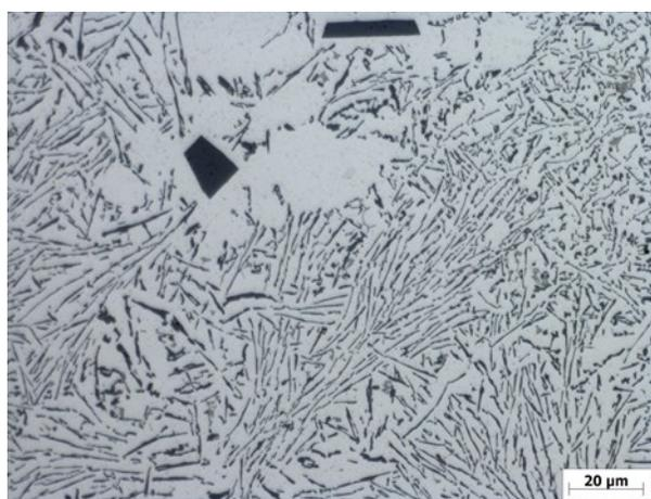
Fig. 8. Microstructure of samples, pressure 150 MPa, temperature 690°C, etched with 0.5% HF
