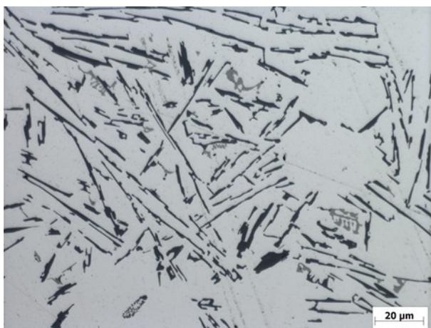
Fig. 4. Microstructure of samples, pressure 0.1MPa, temperature 675°C, etched with 0.5% HF
