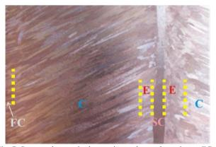
Fig. 7. Structural zones in the continuously cast brass ingot: FC fine columnar, C - columnar, E - equiaxed structure; SC - single crystal (core) situated axially along the ingot
