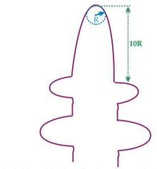
Fig. 4. Definition of the tip radius for columnar dendrites growth (R is the radius of the circle inscribed into the dendrite /cell tip
