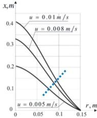
Fig. 8. Localization of the points of inflection (hypothetical localization of the sharp CET) r=0 defines the ingot surface, r=0.15 is connected with the ingot axis; r - distance from the ingot surface (directed to the ingot axis of symmetry)
