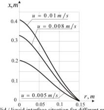
Fig. 6. Solid / liquid interface situation for different rates of the vertical displacement of a brass ingot in the crystallizer
