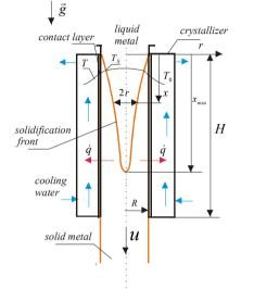
Fig. 5. Model of the system for the continuous casting of brass ingots as shown in the *x*, *r* - coordinates; *Ts*, *TL*- solidus, liquidus isotherm temperature, respectively; *To*- crystallizer average
